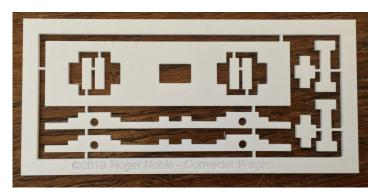
The wagon "fret" was then cut from 1.6mm laser compatible plastic card to create the basic set of components required to form the wagon.
