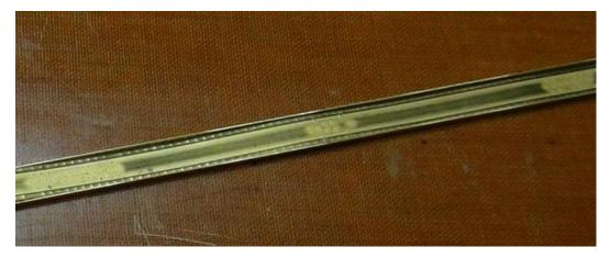
Soldering. First tinning of the beam and the inlay.
