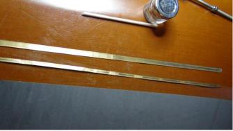
Folding next. The gaps in the fold line made folding so much easier and even though the beam was shuffled along its' length (the Hold n Fold' is shorter), there was no distortion.
