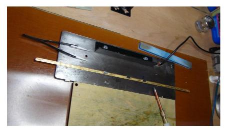
Note the small magnets holding the inlay in place. On this occasion the ceramic tipped tweezers are used edge on (not the tips) to hold the inlay down at the position of the probe contact. This was done with such thin material as using the probe to hold the inlay down would leave a small indentation. The probe position is progressively moved along the beam length.
