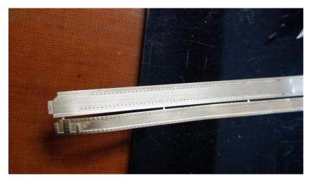
Once the two parts are separated we get the excessive curl, especially on the inlay part which is mostly half etched to 0.1mm thickness.
