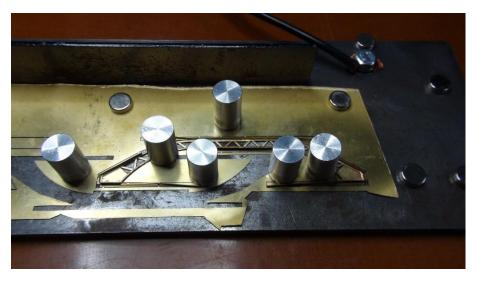
One particular set up was not typical of the usual metal plate or clip to close the circuit. When soldering two parts back to back of a riveted channel section, first the backs were tinned.
