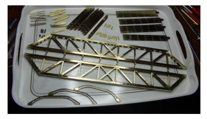
Cleaning up after soldering was done using Flory models sanding sticks, various gravers and finally a good clean with 'Bar Keepers Friend' stain remover
