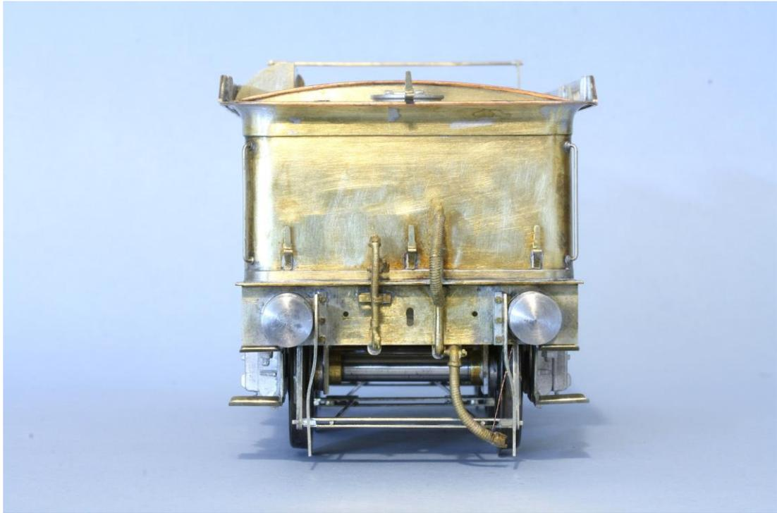
It is also worth taking a closer look at the other end of the tender at the thickness of the fallplate (replaced with 0.010" nickel silver), and the plate that retains the coal which benefits from the addition of fine half round beading to match the detail of the flare.
