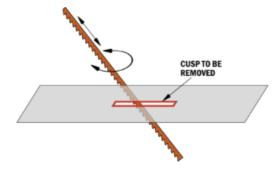
If slots are too narrow, they can be opened with a loose piercing saw blade of matching size. The trick is to pull it through so that the teeth do not cut, but just rub through the slot. Twisting the blade carefully helps. If necessary, repeat with a larger size. This works nicely if the slots have a cusp that needs to be removed.
