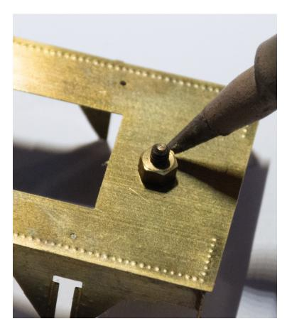
• You should now find the blackened components are free to move, but are firmly held between the head of the pin and the final layer that is soldered to the pin.
