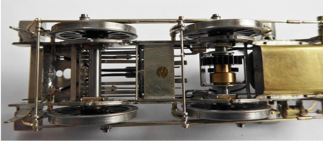
The brake gear is assembled on 0.6mm NS wire, which is both robust enough and springy enough to allow the brake gear to be sprung out of holes in the chassis. Short slices of brass tube are fitted to the 0.7mm brass wire of the hangers, to maintain a constant spacing away from the frame.
