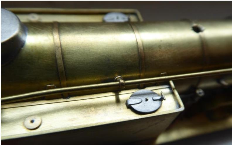
This view also shows the junction of tank top and boiler cladding – again, different to strict MR practice. It appears that there was a narrow flanking strip against the boiler cladding, as well as the pair of trapezoidal riveted brackets; the latter seen here peeking above the ejector pipe run. The dome is still to be fettled; both it and the chimney are whitemetal castings, and will be left till later on before fitting, to avoid accidental damage.
