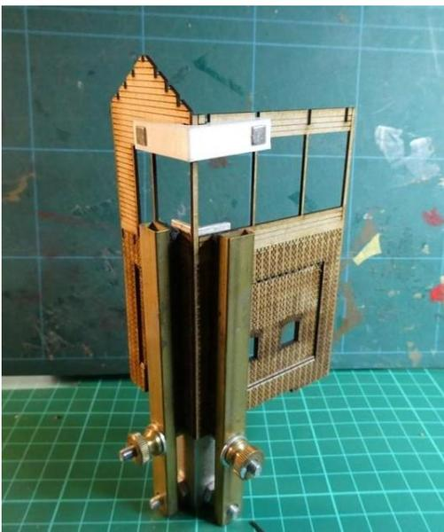
Here two sides have been made up from multiple layers and are being joined using a variety of 90 degree clamps. I used Deluxe innovations Laser Cut kit glue.
