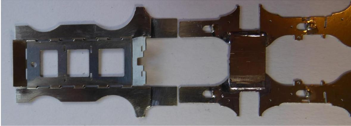
Having completed the solder seams to fix the rear section overlays, the front and rear sections were assembled using Dinky grips, and adjusted over the drawing, to create the necessary 'stretch' between the two elements. Again, great care was taken to avoid introducing any twist at this stage (Pl.6).
