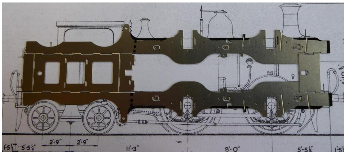
It can be seen how the shortened Rumney chassis 'throws' the brake weigh-shaft and bogie wheel 'arches' forwards by a significant amount. The bogie is thus moved forwards, placing the cab footsteps non-symmetrically to the rear, and so on.
