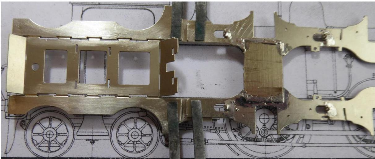
Once the splice-joint soldering had been fully completed, the resultant gap on the inside face was filled with off-cuts from the frame etch. The excess depth of the rear frame overlay, forward of the brake shaft bracket, was filed away, and finally the temporary brace to the front half of the frames was unsoldered and removed, to allow the re-constituted frame to be folded up (Pl.7).
