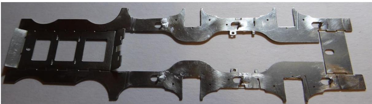
And, to conclude, here is the folded unit prior to soldering the various fold joints, nice and square, with the CSB suspension fulcrum 'ears' folded out and joints reinforced with solder. The front section overlays will then be fitted and their excess depth trimmed off, before the cylinder rear, motion
