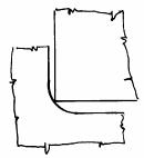
By removing the corner of the bearing hole in the frame by creating a chamfer the bearing will sit against the frame.
