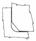
Small castings require their locating holes treated in the same manner to enable them to seat properly. When drilling out holes for fittings the drill will often throw up a burr that prevents the part seating. This MUST be removed. A little cleaning up around the casting spigot may be needed too.
