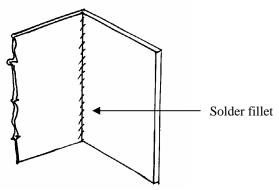
By breaking the corner of the part that has to fit into the corner a better fit can be achieved. Only a small amount of material needs to be removed from the corner. It will not show once the joint is made, as a solder fillet will fill it.
