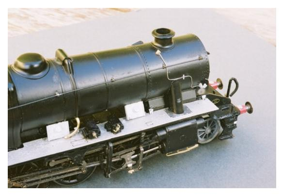
Adding the detailing parts makes a considerable difference to the appearance of this Hornby 8F. They enable basic errors and compromises to be rectified – such as the missing rivets on the running plates, here replaced by etched overlays – as well as allowing the modeller to replicate specific variants within the class.
