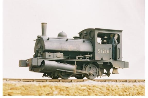
Older RTR models can also benefit from the upgrading treatment. The running of this Dapol 'Pug' has improved out of all recognition by rebuilding it with a new chassis from High Level Kits. The cab area has been opened up and fully detailed but otherwise the body is untouched.
