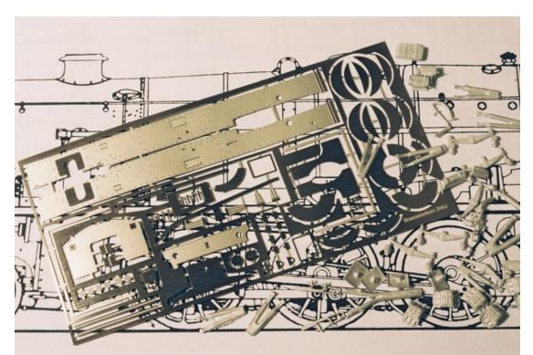
A typical latter-day RTR detailing kit from Brassmasters, with high-quality etched components – a far cry from the lumpy castings of ten or fifteen years.
