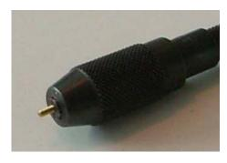
An alternative method of shortening a bush is to put a 10 BA bolt into a pin vice. Set the length protruding to that required on the bush.
