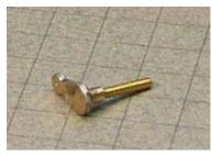
All that remains is to clean up the edges and drill a hole to receive the eccentric rod pivot.
