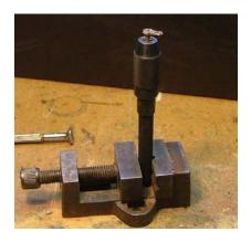
Tin and solder on overlay crank. Holding the parts as illustrated allows the use of both hands. The overlay will often float into position.
