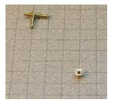
With the same drill countersink the head of the bush. This will allow the bush to screw tightly onto the inner crank.
