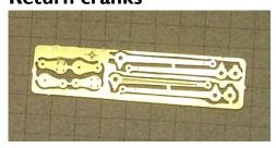
Do all the initial work on the return crank in the fret. It is easier to hold. Illustrated are the inner and overlay
