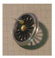
Check assembly of the bush onto the screw. Note the 8BA washer that keeps the rod clear of the wheel face. This washer fits over the bush. Some washers will fit without any adjustment, others will need the hole opening up. I use a round Swiss file as a broach sticks a tries to rotate the washer in whatever you hold it in.
