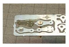
Open up the hole if necessary to 10BA clearance – 1.8mm - in the inner crank Take a larger e.g. 4mm SHARP drill and countersink to accept the countersink of a 10BA screw. The head should protrude slightly above the surface.
