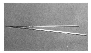
I can now dress the raw vee by draw-filing it in my hand and putting the top radius back. The nose is also blunted slightly. The whole thing is sighted to ensure it forms a true V-shape before I use it. Once we've made our vees they can be cut and trimmed to length and placed on site precisely.
