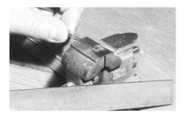
Holding the piece of rail horizontally in the vice, the bend is filed away flat. The rail is then turned over and laid on top of the piece of scrap rail that's already there - the aim is to use this as a guide so you can file off the other piece of rail at the correct angle. The second length of rail for the vee is then put through the same process.
