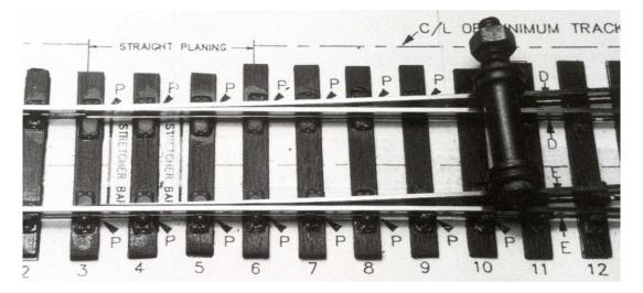
The blade now fits snugly and, since we've already done all the hard work of setting the curved stock rail, it goes in very easily with the help of the gauges. Although it's scarcely visible, I've put a radius on the very tip of the blades so the wheel is guided smoothly into the crossing without any jerks. As long as the blade is tight in against the stock rail, and you're not modelling the Great Western, you don't need any joggle or set in the blade.
