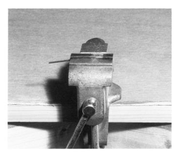
Now comes probably the most important piece to construct the vee. First I place a scrap length of rail into a small smooth-jawed vice at roughly the angle at which I want the vee to end up. Then I take the lengths of rail I want to use for the vee and put a bend 5-6mm from the end in each piece. Remembering that bullhead rail has a top and a bottom, check that the rail is the correct way up and that the bends turn away from each other.
