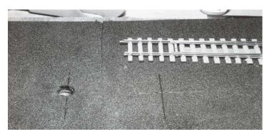
Having marked the exact centre of the tiebar position, I drill a hole straight through the foam and the baseboard. It doesn't need to be the size of the Grand Canyon but this is still quite a hefty hole, maybe around 10mm in 4mm scale, because you need more clearance than you'd think for the operating wire and to allow for any minor adjustments in positioning. Here you can see the locating marks on the right and the hole I've just drilled on the left.
