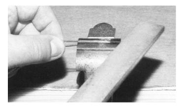
Now I put the vee back in the vice and dress the side where the solder has been used as a filter. At this stage I adjust the angle of the piece of rail in the vice so the top of the vee sits horizontally. This helps in setting up subsequent vees of the same angle.
