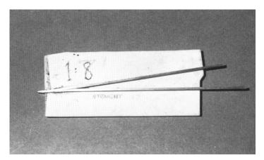
We now see the prepared pieces of rail carefully set up in one of my jigs. I sight them to ensure they form a perfect V shape and do not splay in or out at the end. Then a spot of liquid flux and a touch with the iron, which already has solder on it, makes the joint. I then remove the vee from the jig and spot a little more solder on the side where the two pieces of rail join.
