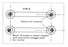
axles centre lines parallel with the track there is no problem, but move one of the centres up or down from the centre line and the rod must lengthen or shorten, and of course, model rods will not. So the holes must be opened out until they run sweetly.
