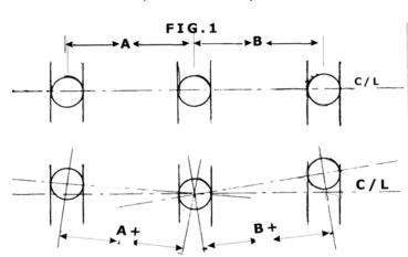
spacers - not unlike our model. But there is a difference, in that the prototype can 'give' slightly as it goes along and our model is absolutely rigid. Secondly, the coupling rods are usually made of a high grade steel, which with only a around 0.002" to 0.003" clearance
