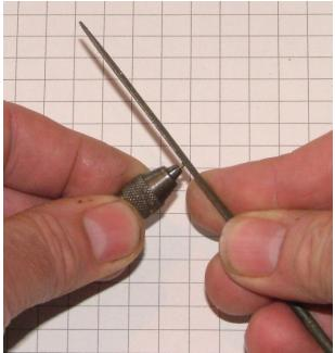
Put the tube back onto the drill and file the tube until the file hits the drill shank.
