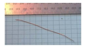
Sometimes thin brass strip will not do the job. Take either fine brass or copper wire (not enamelled) and flatten it. The illustration shows 0.5mm copper wire from telephone cables
