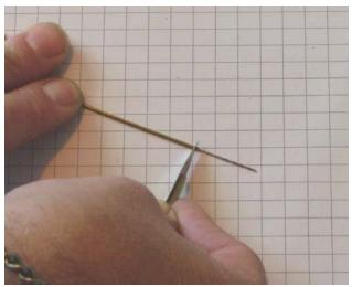
Close to end and slightly longer than needed roll the tube under a scalpel blade. This will either cut through or at least score the tube. Draw the drill out until the end is nearly under the cut and use it as a lever to break off the short length. This also serves to stop the cut piece from being lost!
