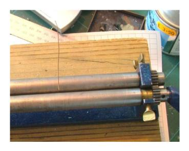
Here the wire is passing through the rolling bars. Copper will go through without annealing, brass needs it.
