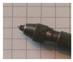
To get the final length insert the drill in a pin vice with drill shank protruding. Set the length required and tighten the chuck.
