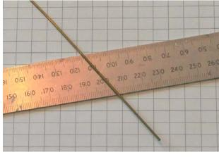
Small bore brass tube to be cut into short lengths.
