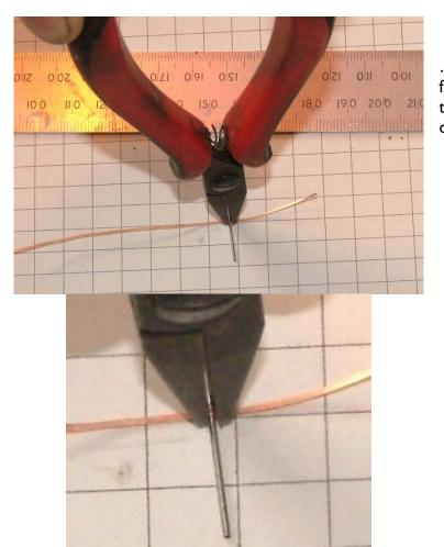
... press a pair of plain flat pliers over the wire to deform it over the drill.
