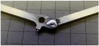
The joint should still be free after soldering.. Clean up the solder nearly flush with back of the
