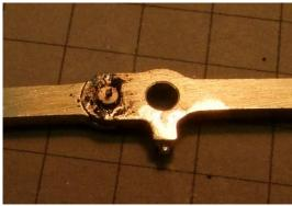
In this case the pin has an unusually large parting-off pip. This can be easily removed with a few strokes of the file. Leave in the joint whilst you do this; it makes a convenient handle and will prevent it disappearing.
