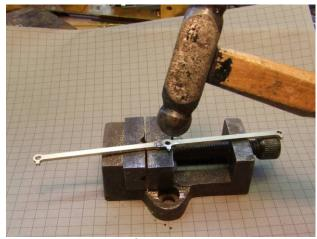
Use the ball pein of a hammer to set the end of the pin. The head of the pin is on a suitable anvil. The end will be expanded into the countersink.
