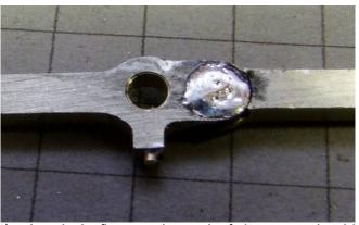
Apply a little flux on the end of the pin and solder with 188 solder.
